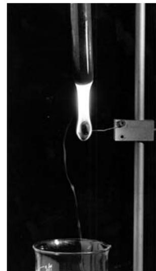
1. Bend the large paper clip to make a peanut holder. Use tape to mount the paper clip in the center of the aluminum plate (pie pan). The pie pan is necessary because the burning peanut may fall off the holder or drip flaming fat drops.
